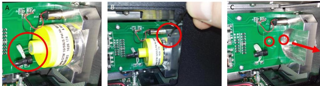
Figure 47: Remove light bulb.
