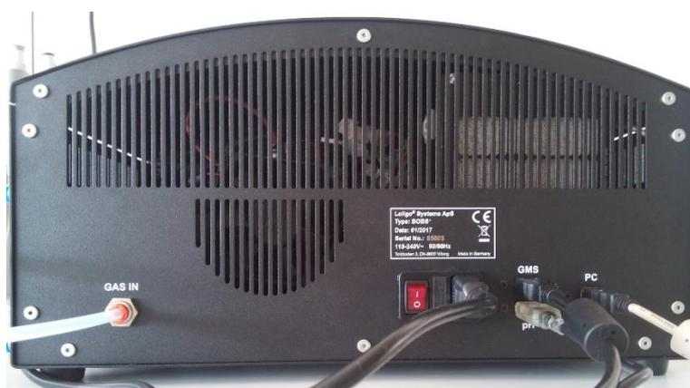
Figure 7: Rear connections
