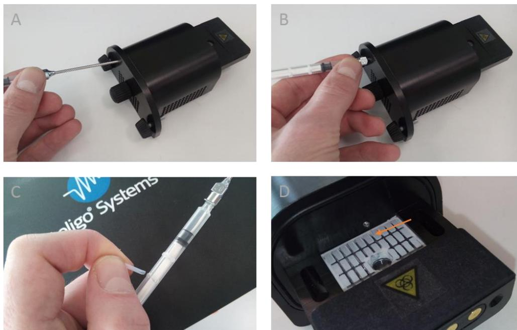
Figure 10: Insert pH microsensor.
