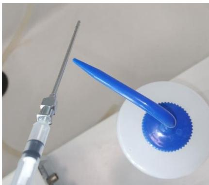
Figure 18: Cleaning of pH sensor
