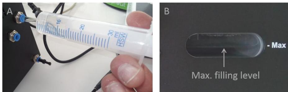
Figure 6: Filling the water reservoir.
