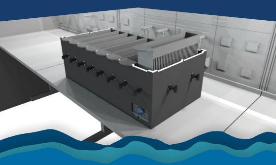
Automated CT<sub>Max</sub> systems for exact temperature control and efficient handling and exposure of multiple animals
