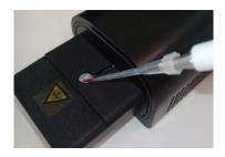
**NOTE:** If you are not using the pH-sensor, the entrance port for the pH sensor inside the sample holder must be covered with a small piece of tape to avoid air draft and any condensation forming inside the pH sensor tube to run back into your sample and dilute it.
