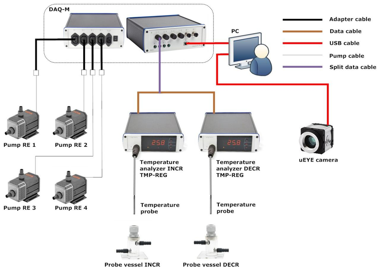
**Figure 1:** How to connect the temperature instruments (TEMP-REG), temperature probes, temperature regulation pumps (RE pumps) and uEye camera for running a ShuttleBox temperature experiment.
