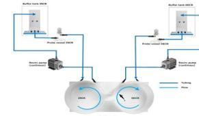
7. Place the coils in heating/cooling baths and connect them to the pumps and the buffer tanks.
