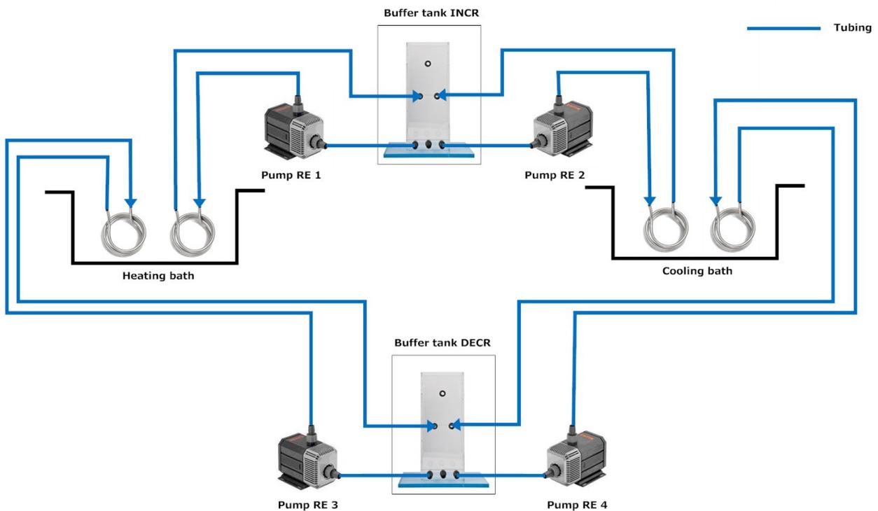
**Figure 3:** How to connect the buffer tanks with the cooling and heating baths (not supplied) for running a ShuttleBox temperature experiment.
