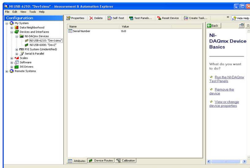
Now change the device name of the NI USB-6008 DAQ card to "dev1". The DAQ-S instrument should now work properly with ShuttleSoft.
