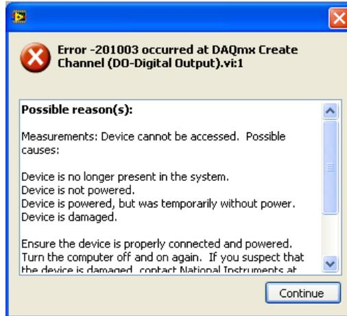
The error shown in the screen above occurs, when the NI-USB 6008/6009 DAQ card is not properly connected to the PC. This error can occur in 2 ways.
