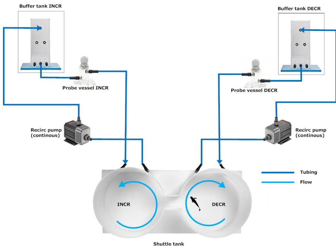
**Figure 2:** How to connect the Shuttle tank with the recirculation pumps, buffer tanks and temperature probe vessels for running a ShuttleBox temperature experiment.
