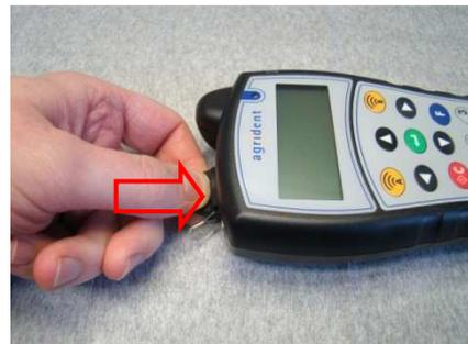
When you connect the APR500 to a particular PC via USB the first time, Windows will detect the new device automatically and ask for a driver. Please choose to install the device manually and use the APR500.inf file from the APR product CD. For a more detailed description please read the separate driver installation guide.
