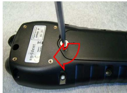
Put the battery cover back in place and turn the screw 90° clockwise. Be aware, that the APR500 housing will only retain its protection class when the battery cover is properly attached.
