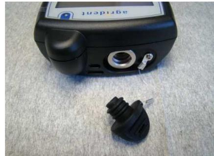
Please be aware that the male APC connector has two noses and the plug in the reader has two notches, the position of both has to match.
