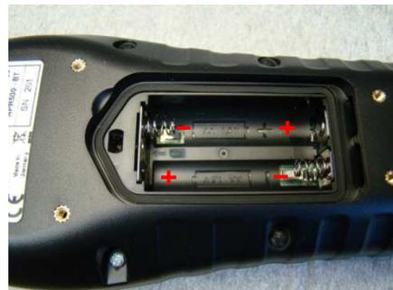
Remove the battery cover and then the batteries. Please pay attention on the imprinted battery symbols in order to insert the batteries in the correct direction. Use only AA standard or rechargeable NiMH cells, but note that only Agrident supplied rechargeable batteries can be charged internally.
