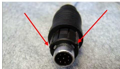
If the connector of the APC and the plug in the APR are mated correctly, push the connector until it snaps into place noticeably. Now connect the USB-A connector resp. the 9-pin RS232 connector into the corresponding plug of the device you want to communicate with in order to complete the connection.
