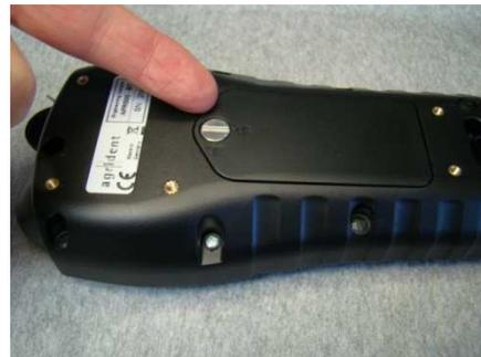
Turn the screw of the battery cover 90° counter clockwise. You might use a screwdriver or a small coin for that. Lift the lid by using your fingernail or an appropriate tool.
