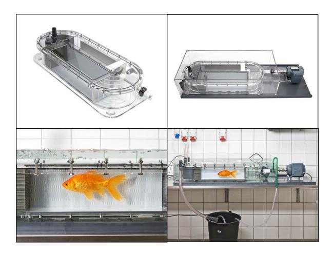
The unique and compact design allows adequate space for movements and at the same time a minimum footprint and a low volume required for reliable oxygen consumption measurements.
