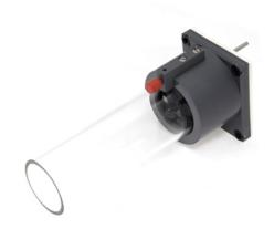
3. Insert the inner glass tube into the outer one. The honeycomb section should end up right next to the propeller.
