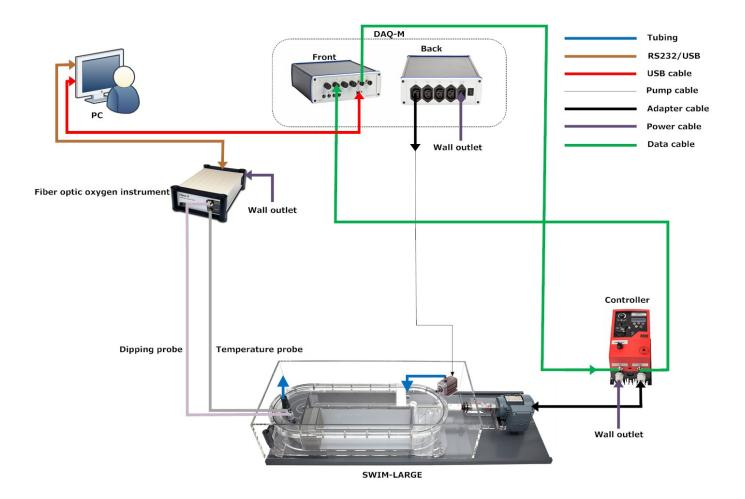
Please see below for a diagram depicting full set-up of large swim tunnel with OXY-REG instrument and galvanic electrode (supplied separately).
