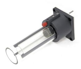
4. Then push the other end cap over the end of the outer tube. The two screws in the mounting bracket at the floor of the ambient tank should fit the lower holes in the end cap.
